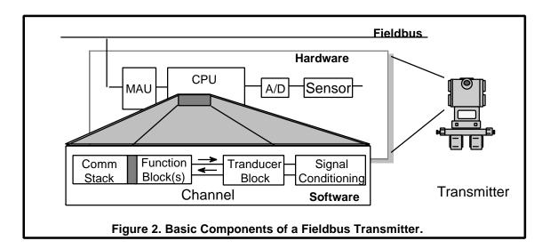
Figure 2 illustrates a similar architecture for a transmitter. In this case the TB interfaces with the signal conditioning circuit of the sensing device, which is manufacturer specific. Then, via a numbered channel, connects to an Analog Input (AI) function block. The AI block has 36 standard parameters. It provides a scaling function, filtering, and process and block alarms. The simulate parameter is provided, as in the AO block, for test purposes.
