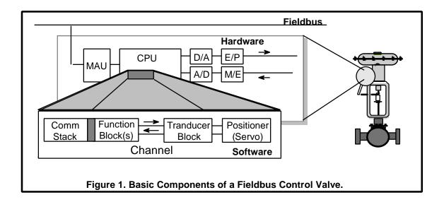
Figure 1 illustrates the key hardware components in the background, and software is shown as a projection from the CPU's memory. Considering the hardware first, MAU stands for Medium Attachment Unit and comprises the circuit needed to connect the device to the actual bus wires. The device will have a microprocessor, indicated here by the shorthand, CPU.
